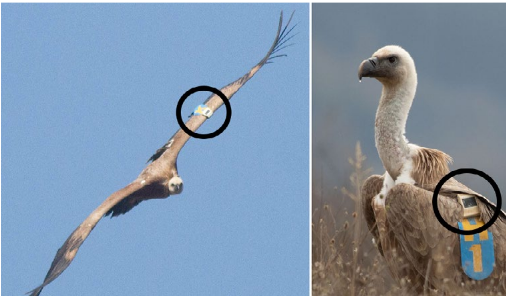
Figure 4. Patagial GPS/GPRS transmitter OT-P33 mounted in griffon vulture – left- in flight; right – landed.
